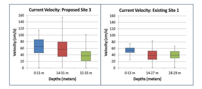
Figure 5. Box and Whisker Plot showing extreme ranges of current velocity (thin vertical lines), 50% of observations (25% each in the colored boxes) and the average flow (as the thin black horizontal line in the colored boxes). Proposed Site 3 plot from raw data, existing Site 1 plot reflects adjustments to make the time period comparable to Site 3 as explained in the narrative.
