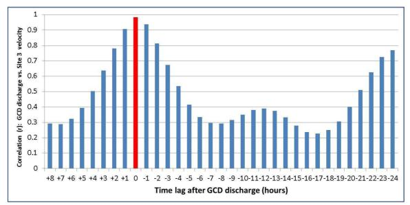
Figure 3. Time lag before and after Grand Coulee Dam (GCD) discharge and current meter measurements in the top 12 meters at proposed Site 3 in Rufus Woods Lake and correlation coefficient (r).
