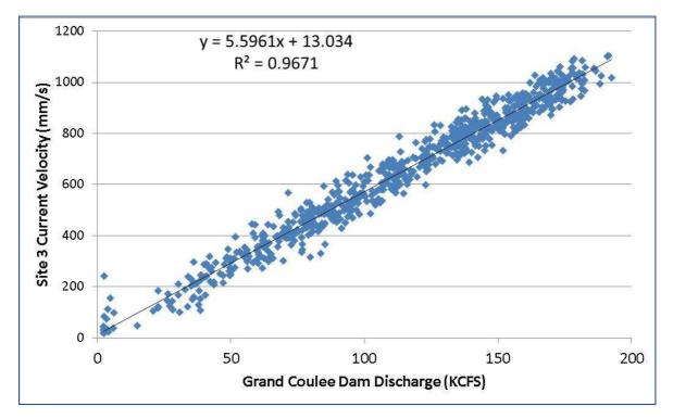
Figure 4. Site 3 water current velocities in top 12 m of the water column versus simultaneous hourly mean discharge at Grand Coulee Dam in the pertinent time periods discussed above. Coefficient of determination ( $R^2$ ) and linear equation shown.
