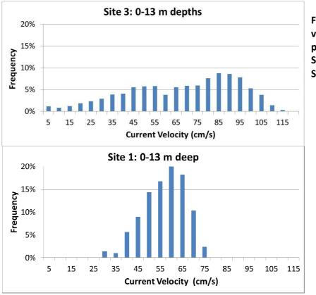
Figure 6. Current velocity frequency plots at proposed Site 3 and existing Site 1.
